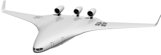
Fig. 12 View of the silent aircraft lower-risk design.
